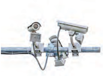
Analog CCTV System transmit video over coaxial cables to a digital video recorder (DVR)
